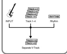
In the following example, we'll assume that tracks 1 and 2 contain mono recordings and tracks 3 and 4 contain a stereo-recorded performance, and you want to bounce-record all of these to V-track 2 of tracks 3/4.
