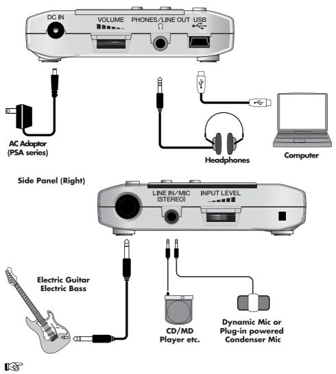
Plug-in powered microphone (p. 18)
