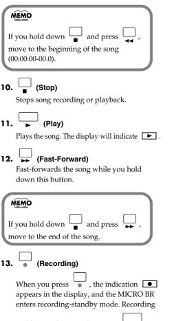
will begin when you then press  $\$  . In addition to recording operations, this button is also used to perform punch-in/out operations.
