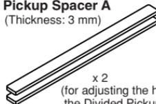
x 2 (for adjusting the height of the Divided Pickup)
