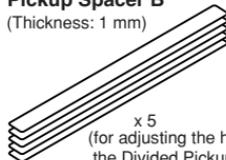
x 5 (for adjusting the height of the Divided Pickup)
