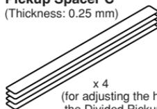
x 4 (for adjusting the height of the Divided Pickup)
