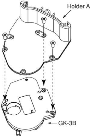
\* Holder A has six screw holes. Refer to the figure to ensure the holder is attached correctly.
