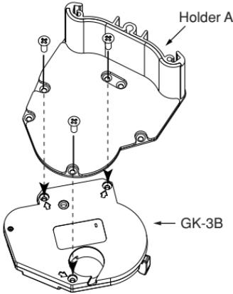
\* Holder A has six screw holes. Refer to the figure to ensure the holder is attached correctly.
